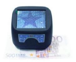
The HS3B Forensic Magnifier is a simple to use battery and mains operated magnifier with 8 integrated light sources for rapid authentication of ID cards, passports, currency and for visualising fingerprints. The magnifier has an integrated CMOS camera and 3 inch TFT screen for displaying the images. Images can be stored, compared and exported.
